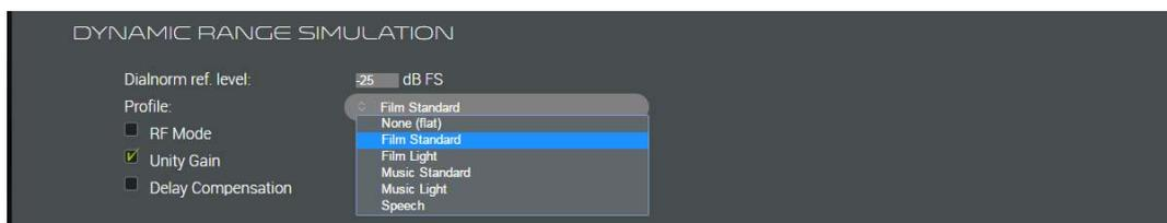
These parameters are applied whenever the **DRC** button on the **CONTROLLER** page is selected, see 7.1.7: *Dynamic Range Compression (DRC)*. The simulation complies with the SMPTE 85 standard used in Dolby encoding:
