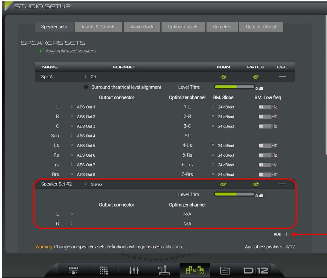
The screenshot shows the 'STUDIO SETUP' interface with the 'SPEAKERS SETS' section active. The interface includes a table of speaker sets and an 'ADD +' button. A red box highlights the 'Speaker Set #2' entry, and a red arrow points to the 'ADD +' button with the text 'Click here to ADD a new speaker set'.
