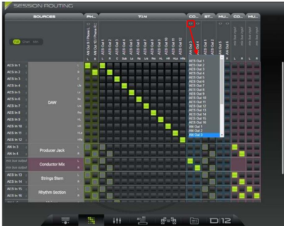
The I/O assignments of all sources and destinations can be adjusted except for the speaker sets (as their I/O assignments are part of the **STUDIO SETUP** rather than the **SESSION SETTINGS**). See *STUDIO SETUP -> Speaker Sets*.
