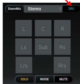
The **DRC** button in the **SPEAKERS** area can be used to simulate how your mix will sound when played through a consumer system (where dialogue normalization is applied).
