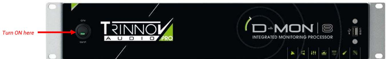
You will hear a click from the internal relay, and the **ON** button illuminates as shown above. The processor will take a few seconds to boot, so please wait a little while before opening the GUI.
