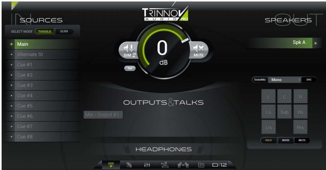
The GUI is optimized for 4:3. Therefore, please adjust your browser's window size and screen resolution accordingly. You should now be able to see all parameters clearly - in our example, the headphones **ON/OFF** button, source select and volume.
