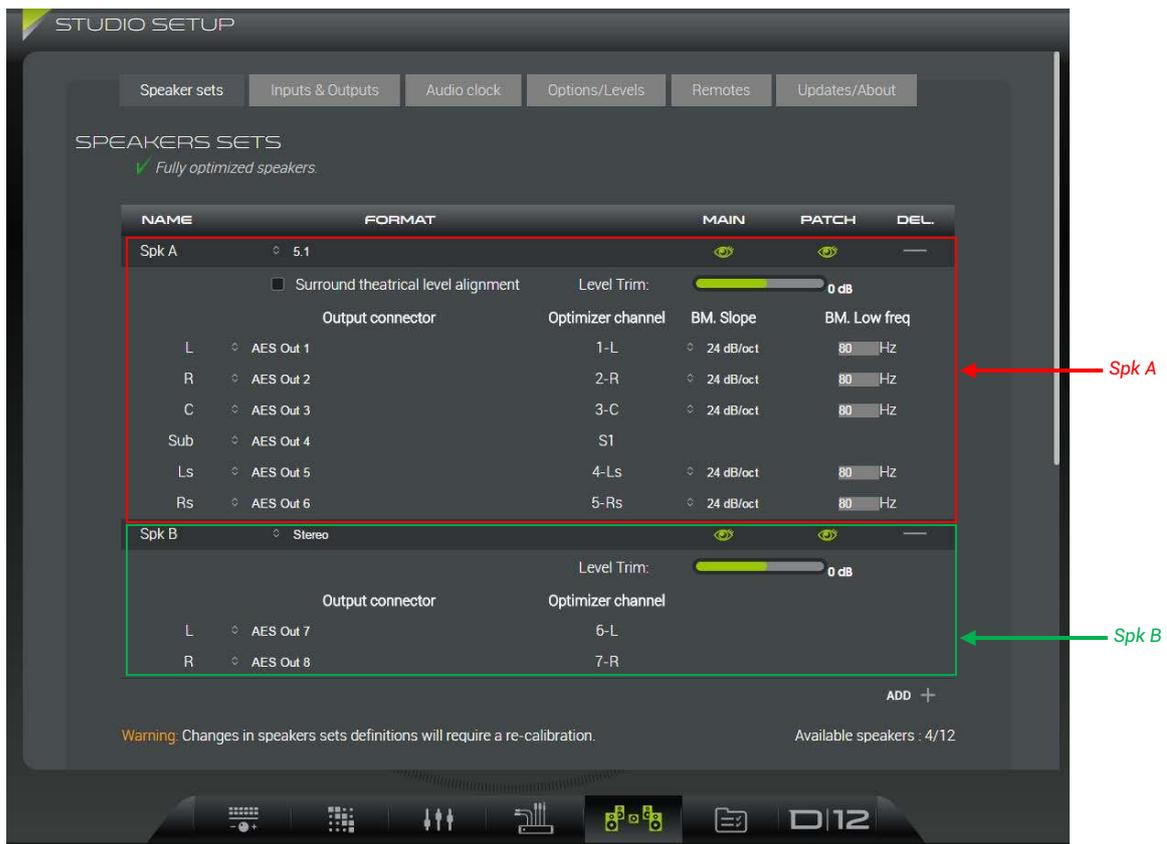
The screenshot shows the 'SPEAKERS SETS' configuration page. It features a table with columns for NAME, FORMAT, MAIN, PATCH, and DEL. Two speaker sets are listed:
