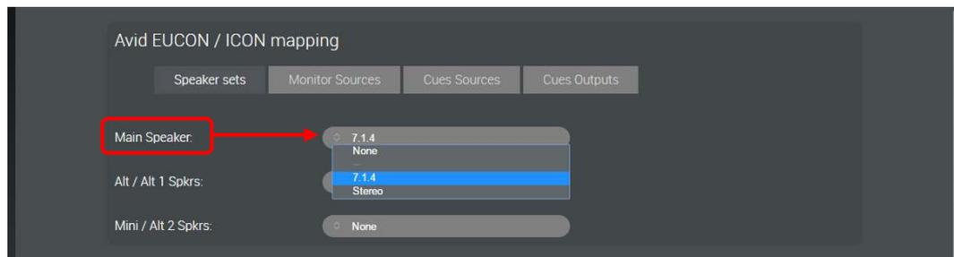
The external controller functions are pre-determined by the connection protocol (either Avid EUCON or ICON). The available resources depend on the D-Mon processor configuration; in our example above, two speaker sets have been defined (in the *STUDIO SETUP -> Speaker Sets*) and, therefore, either of these can be assigned to the function **Main Speaker**.
