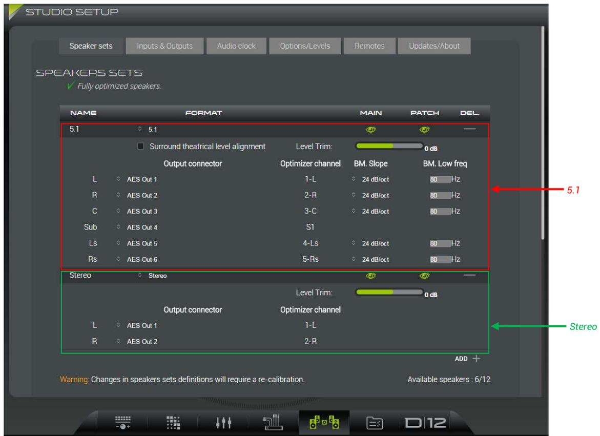
In this example, there are still two speaker sets, but this time the Left and Right channels connect to the same physical outputs and, therefore, can share the same Optimizer channels (1 & 2).
