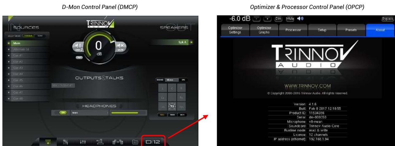
The **Optimizer & Processor Control Panel (OPCP)** is a lower-level interface to the D-Mon processor than the DMCP GUI. Use the page buttons running across the top of the GUI to access its pages (e.g. **Optimizer Settings**, **Optimizer Graphs**, etc.).
