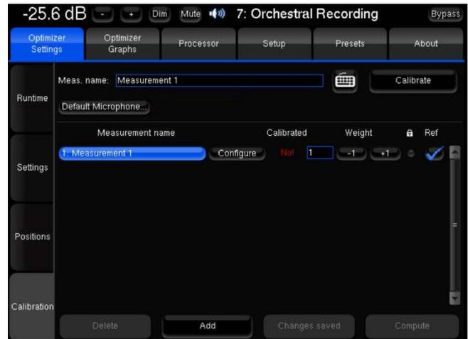
5 Click on **Calibrate** to start the calibration procedure, and follow the on-screen instructions:
